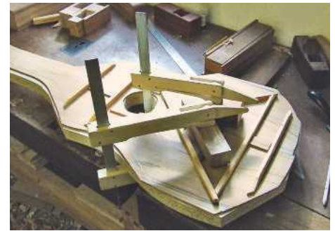
▲ Pic.6 Glue on the braces – start with the graft between the cross braces to provide positive location. Cauls and long-reach clamps are necessary to get proper clamping pressure
